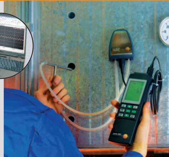
Pitot tube measurement with external 100 Pa probe
