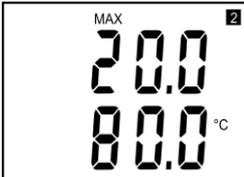
After next press of the button value for upper point appears, here 20 mA corresponds to ambient temperature 80 °C.
