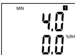
Range and type of value for output 1 (current loop I1 = symbol „1“ on display). Type of value, assigned to output 1, is indicated by displayed unit (here %RH = relative humidity). Upper line displays current value corresponding to measured value (lower line). Here 4 mA corresponds to 0%RH.
