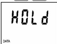
Press ENTER key to display values stored in the HOLD memory. Press DISPLAY key to display other stored values (dew point temperature). Press MENU key to leave this mode.
