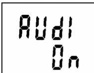
This item indicates if audio signaling of alarm indication is switched on (On) or switched off (OFF). Press ENTER key to change actual setting. Notice: if the battery voltage is low, audio indication is out of operation to reduce current consumption independently on this selection.
