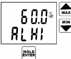
Reading ALHI indicates adjusted upper limit of the same alarm (here air temperature). Set the desired value in the same way as in above lower limit. If needed it is possible to get back to lower limit setting of the same alarm by pressing DISPLAY key. Press ENTER key to confirm new upper limit.
