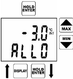
Reading ALLO indicates adjusted lower alarm limit (here air temperature). Set the desired value by means of the arrow keys. Press and hold the arrow key UP to make value increase fast. Press and hold the arrow key DOWN to make value decrease fast. Release the arrow key and press ENTER to confirm new limit.
