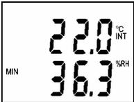
Switched ON instrument permanently updates minimum and maximum memory of each measured values. Press MIN key (resp. MAX key) in the default mode to display minimum (resp. maximum) reading. These minimum and maximum readings are indicated by MIN (MAX) symbols on the LCD. Press DISPLAY key to display minimum (resp. maximum) value of other values.
