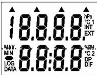
If you wish to use the external temperature probe, connect it before instrument switching ON. Switch ON the instrument by pressing ON/OFF key. After switching ON the instrument all symbols on the LCD are displayed. If the ON/OFF key is being held pressed, all LCD symbols are displayed till the key is released.
