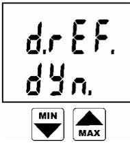
Display refresh mode is indicated. In the FAST mode refreshment is fastest with regular interval approximately 0.7 s. In the dynamic refresh mode (DYN.) each 15 s refresh interval of display is doubled to maximum 5 s if measured values are stable. If measured values change, refresh interval decreases to approximately 0.7 s. This dynamic mode prolongs battery life significantly. Select the desired mode by ENTER key.
