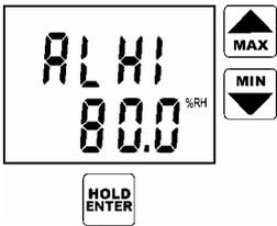
Instruments further offers alarm setting of other measured quantities. It is possible to leave the alarm setting mode by pressing MENU key. New adjusted limits up to pressing MENU key are stored in memory. After pressing ENTER key it is possible to set alarm limits for dew point temperature.
