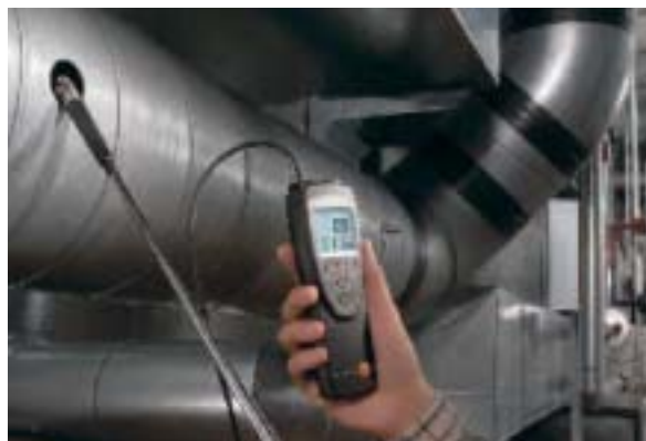
testo 416, e.g. for monitoring the volume flow of the exhaust air
