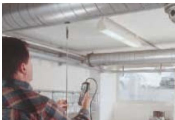
testo 416 e.g. for setting the air input in a kitchen
