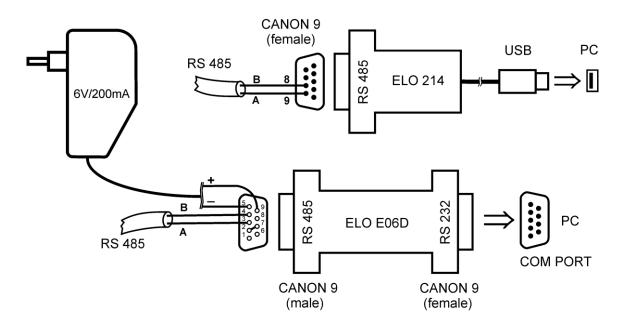
The ELO E06D converter is an optional accessory for connection of transmitter with RS485 interface to the PC via serial port RS232. Connect connector marked RS232 directly to the PC, connect power to connector marked RS485. Power voltage +6V DC from an external acdc adapter connect to pin 9, 0V connect to pin 5. Also mutually connect pin 2 and pin 7. Link RS485 is connected across pin 3 (A+) and pin 4 (B-).
