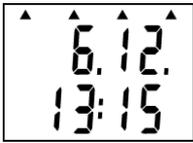
If battery voltage drop occurred since last internal clock setting below critical limit or battery disconnection for longer period than approximately 30 s, after display switch ON (during date and time display) all four arrows appears as warning to check or set it again from the computer. However all logger functions work without limitation.
