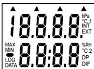
After switching ON the logger all LCD symbols are displayed for checking the display.
