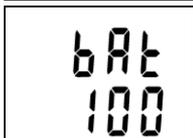
Consequently reading of estimated remaining battery capacity for approximately 2 s is displayed (values 0 to 100%).
