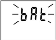
If reading BAT is displayed periodically on LCD upper line (for 1 s with 10 s interval), the end of estimated battery life is coming – however logger functions are not limited. Replace battery as soon as possible!
