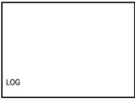
If display is switched OFF, all above readings are displayed up to estimated remaining battery capacity and then display goes out. If logger is switched ON symbol LOG is displayed (it blinks if memory occupation is higher than 90%).
