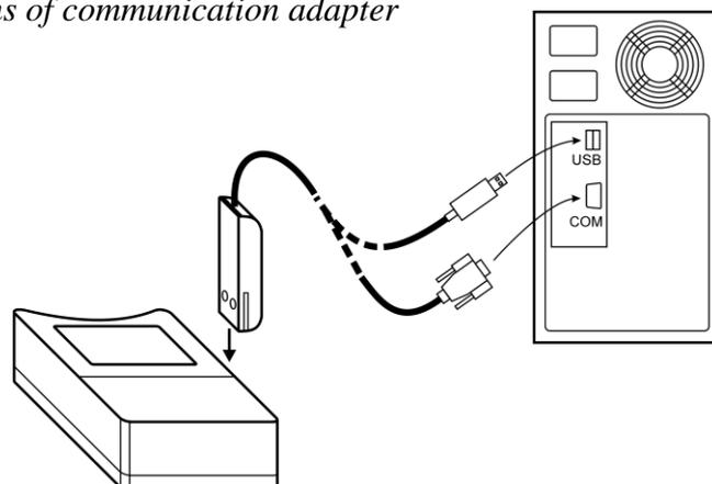
**Notice:** USB connector can be located also from the computer front side
