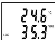
**If display is switched ON**, actual reading of measured values is displayed - ambient temperature (°C) on the LCD upper line, relative humidity (%RH) on the LCD lower line. Symbol LOG indicates data logging in progress – if it blinks, data memory is filled up to more than 90%.
