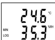
Switched ON logger permanently (with 10 s interval) updates memory of minimum and maximum values of each measured (or calculated) quantity. If displaying of MIN/MAX values is selected, minimum measured values are displayed step by step (indicated by symbol MIN) and then similarly maximum measured values of all quantities (indicated by symbol MAX). The entire cycle is repeated periodically, i.e. reading of actual measured values follows.
