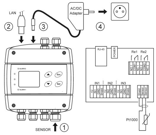
Binary inputs are not galvanic isolated, connection terminals +U are internally connected to the device power supply (ie. the +U terminals provide the same voltage level as power supply).
