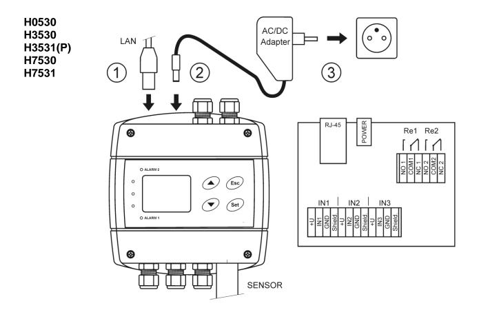
Binary inputs are not galvanic isolated, connection terminals +U are internally connected to the device power supply (ie. the +U terminals provide the same voltage level as power supply).
