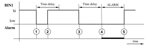
A figure shows a simple example. Binary input 1 is configured to send an e-mail if input change state from high to low (lower edge). At point 1 a binary input was opened. Because at point 2 input was closed before the time delay expired, alarm was not set. At point 3 was input opened again. At point 4 the time delay expires and at this moment e-mail, SNMP traps are sent. The alarm lasted to point 5, where the input was closed.
