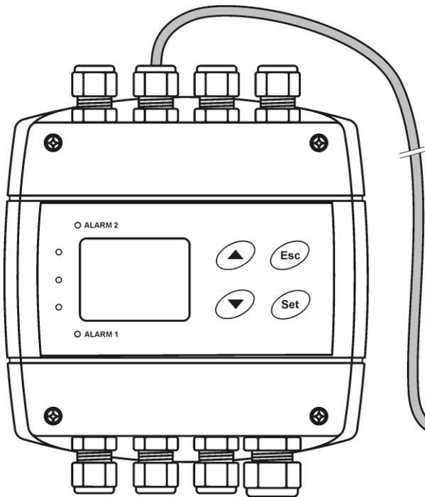
**GPRS modem** is intended for wireless transmission of actual measured values from regulator. In the event of alarm state, the user is informed by the SMS message. In places, where communications networks are missing, the GPRS modem enables on-line data acquisition.
