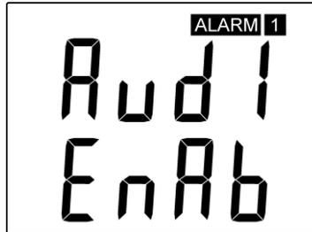
**Acoustic alarm assign to relay 2**
