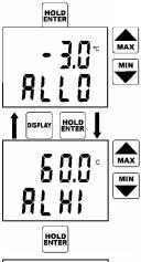
Reading ALLO indicates adjusted lower alarm limit (here air temperature). Set the desired value by means of the arrow keys. Press and hold the arrow key UP to make value increase fast. Press and hold the arrow key DOWN to make value decrease fast. Release the arrow key and press ENTER to confirm new limit
