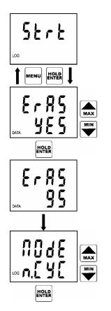
If it is needed to clear the memory before logging start, first it is necessary to select menu item logging START (symbol Strt) and confirm by pressing ENTER key.
