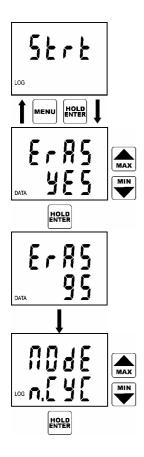
If it is needed to clear the memory before logging start, first it is necessary to select menu item logging START (symbol Strt) and confirm by pressing ENTER key.
